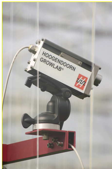
The GROWLAB Plant temperature camera measures the temperature of the plant using infrared.
