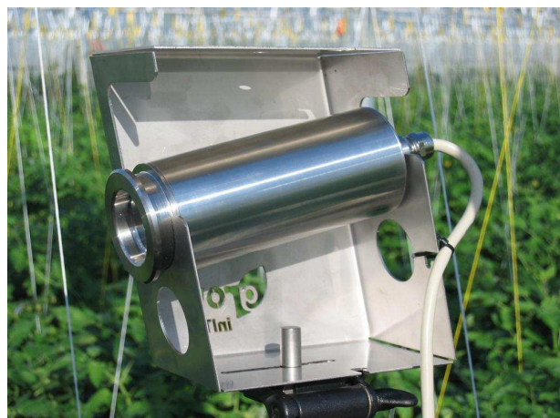
Illustration 6a - Plant temperature camera
